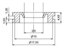
The shaft seals specially manufactured by SEC are perfectly suited for applications with our VISEC rotor units of the D-series. Installed in the seal housing, they ensure a smooth metering process, without leaks.
