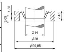
The shaft seals specially manufactured by SEC are perfectly suited for applications with our VISEC rotor units of the R-series UR8 und UR10. Installed in the seal housing, they ensure a smooth metering process, without leaks.
